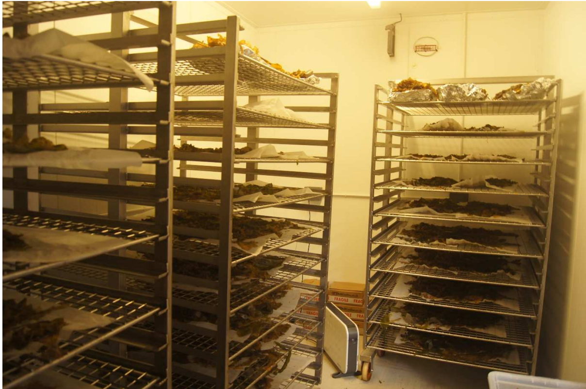
Fig 24. NAFC Marine Centre's dedicated seaweed drying room: a redundant walk-in freezer fitted with drying racks, dehumidifiers, heaters, and fans.
